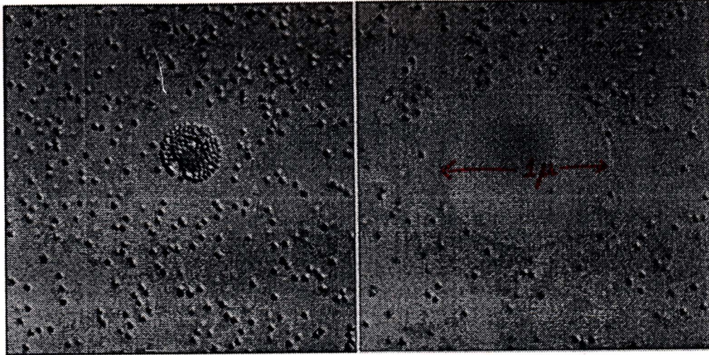
Fig. 1. A self-limited array of latex spheres on a charged surfactant vesicle at room temperature (3). The spheres are on the surface of a vesicle viewed in differential interference microscopy, focusing on the array itself (left) or on the vesicle equator (right). The membrane is a mixture of cationic and neutral surfactants (DDAB and Triton X, respectively, with octanol added to stabilize bilayer structures). The sphere diameter is 1 μm ; the sphere volume fraction is 0.004.
