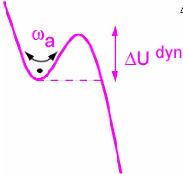
$$\Delta U^{dyn}(I_0, i_{RF}, \alpha) = \underbrace{\left[ \frac{64\hbar}{18e\sqrt{3}} I_0 \alpha (1-\alpha)^3 \right]}_{u_0^{dyn} \approx 10\text{K}} \left( 1 - \left( \frac{i_{RF}}{I_B} \right)^2 \right)^{3/2}$$
