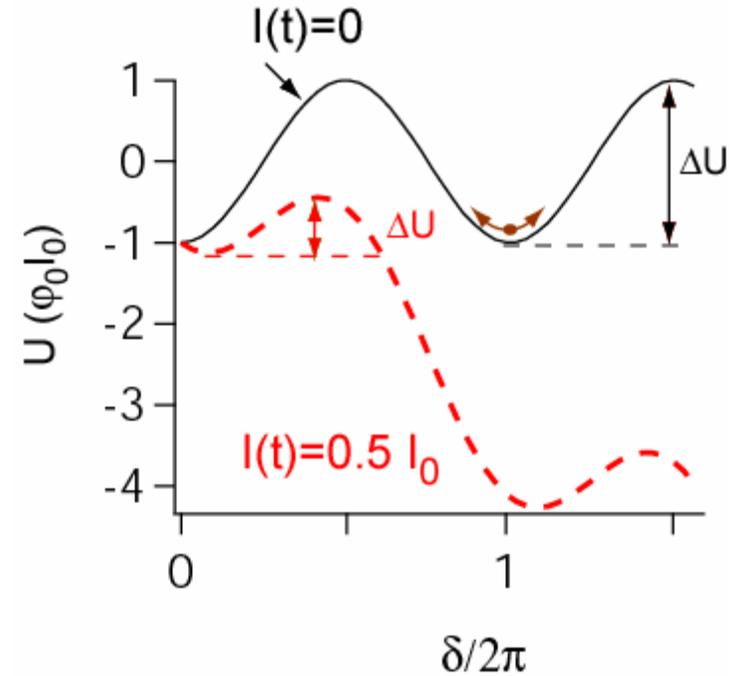
$$\Gamma_{0 \rightarrow 1}(I_0, I_{DC}, T) = \frac{\omega_p}{2\pi} \exp\left(-\frac{\Delta U}{kT}\right)$$
