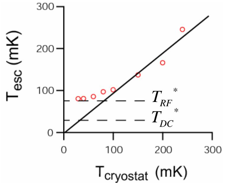
$$T_{RF}^* = \frac{\hbar\omega}{k}$$
