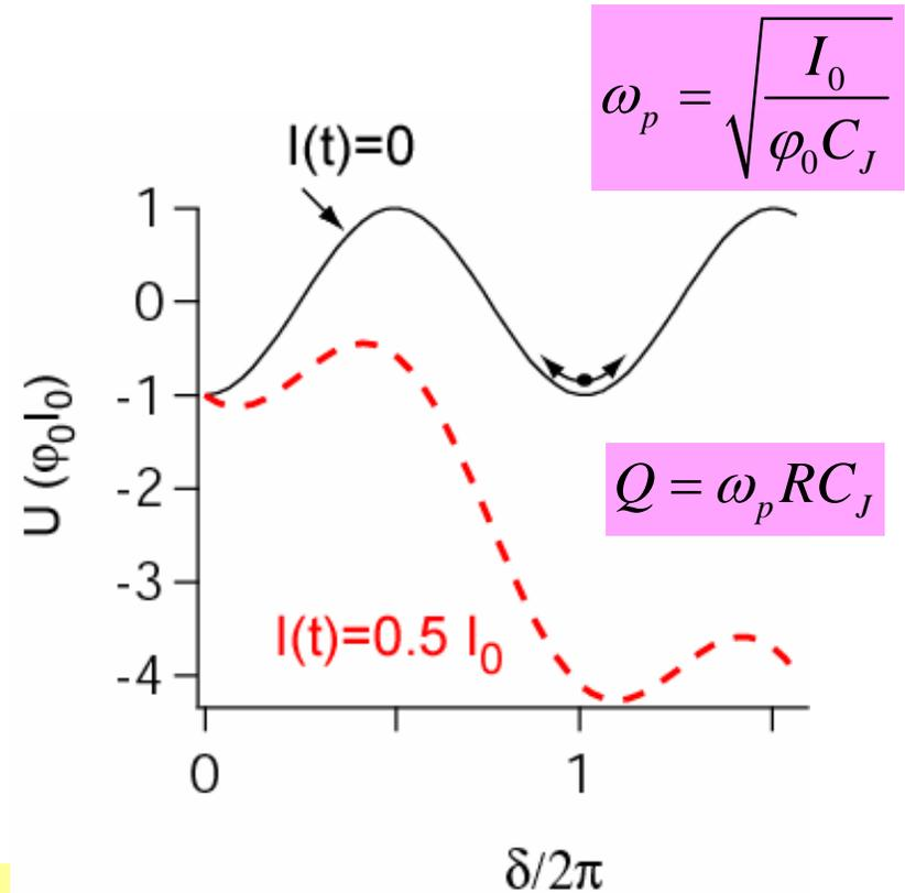
$$\underbrace{\varphi_0^2 C_J}_{\text{mass}} \frac{d^2 \delta}{dt^2} + \underbrace{\frac{\varphi_0^2}{R}}_{\text{drag}} \frac{d\delta}{dt} + \underbrace{\varphi_0 I_0 \sin \delta - \varphi_0 I(t)}_{\frac{\partial U(\delta)}{\partial \delta}} = 0$$
