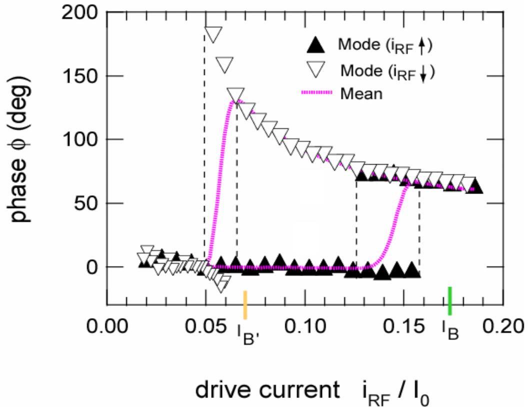
$$I_B = \left[ \frac{16}{3\sqrt{3}} \alpha^{3/2} (1-\alpha)^{3/2} \right] I_0 \quad \alpha = \left( 1 - \frac{\omega}{\omega_p} \right) = 0.122$$
