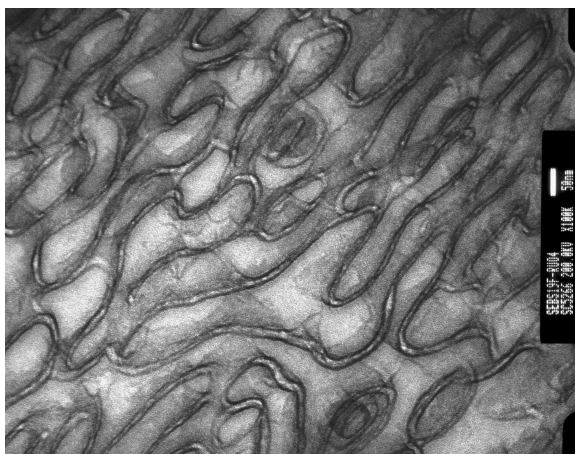
Figure 19: PSEBS-in-PS sponge, realized for PSEBS volume fractions greater than about 0.20 and less than about 0.4.
