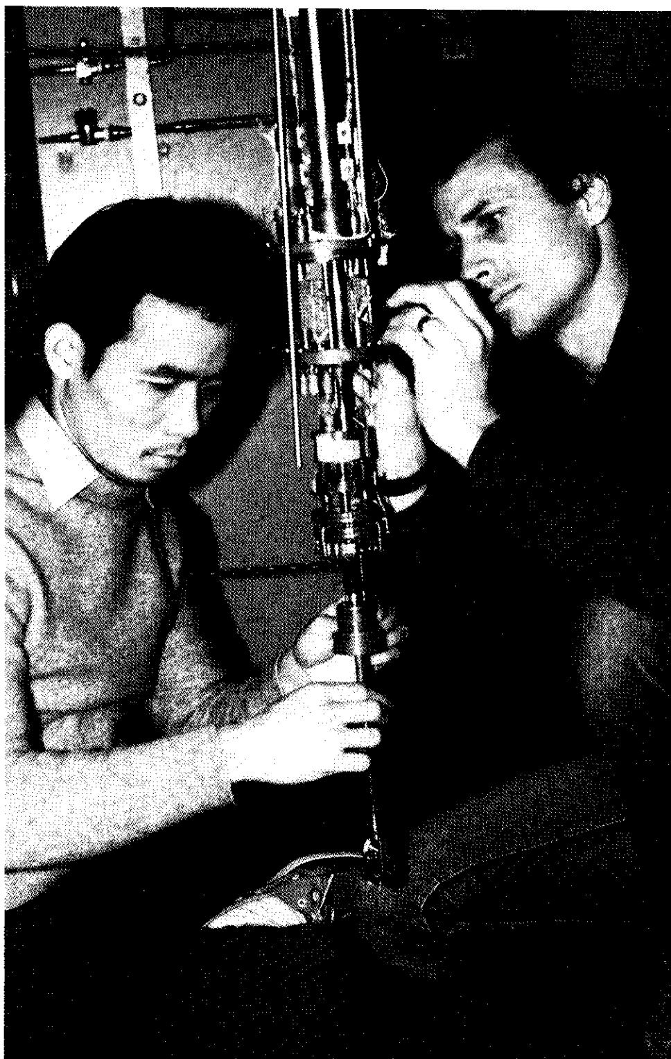
Dilution refrigerator for cooling f -electron materials to millikelvin temperatures. Here graduate student Jenq-Wei Chen and postdoctoral research physicist Steven Lambert prepare the \text{He}^3\text{-He}^4 refrigerator for measurements of the upper critical magnetic fields of heavy-electron superconductors. Figure 1
