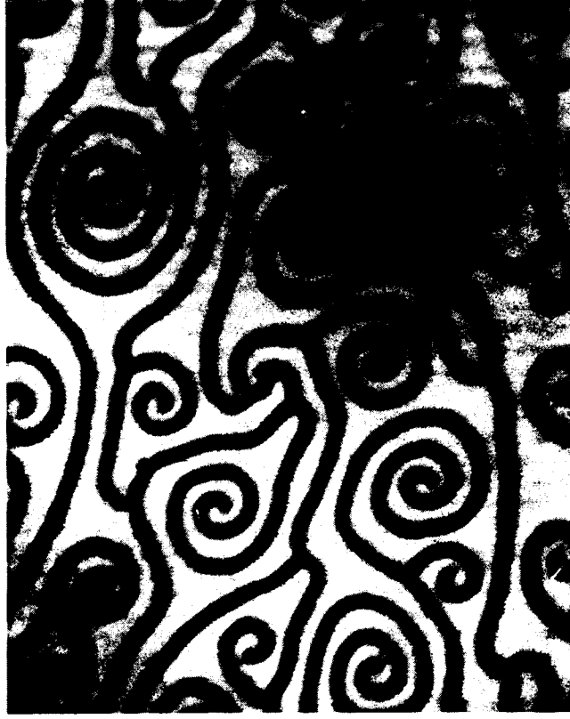
Fig. IV-39. Epifluorescence photomicrograph of crystalline domains of a dipalmitoylphosphatidylcholine monolayer containing 2% cholesterol and compressed to the plateau region. From H. M. McConnell, D. Keller, and H. Gaub. Phys. Chem. , 90 , 1717 (1986). Copyright 1986, American Chemical Society.
