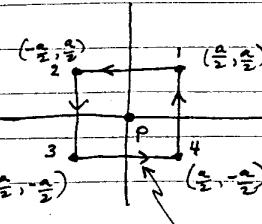
Let the contour  $C$  be the perimeter of the "plaquette" shown in the figure. Then  $\hat{n}$  is a unit normal pointing out of the page. Now take the area  $A$  to zero (i.e., take  $a \rightarrow 0$ ); then
