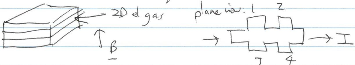
$$\text{resistance } R_{xx} = \frac{V_{12}}{I}, \quad R_{xy} = \frac{V_{13}}{I}$$
