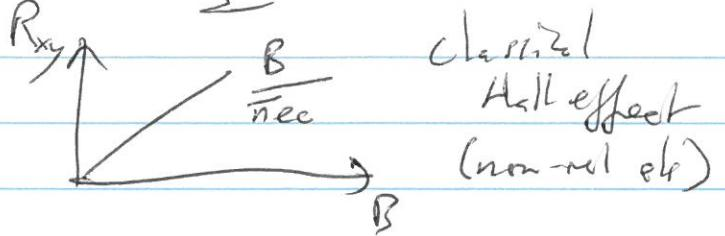
$$\text{Classically (clean system)} \quad R_{xy} = \frac{\sigma_{xy}}{\bar{n} e^2} = \frac{B}{\bar{n} e c} = \frac{B}{\bar{n}} \cdot \frac{e}{h c} \cdot \frac{h}{e^2}$$
