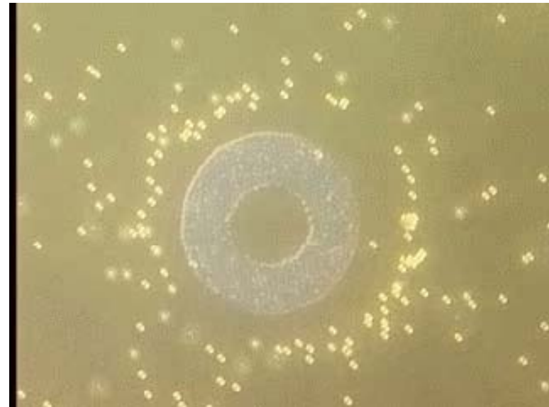
Real-time pattern formation of 1 \mu\text{m} polystyrene spheres on Ag patterned gold surface at 500x*
