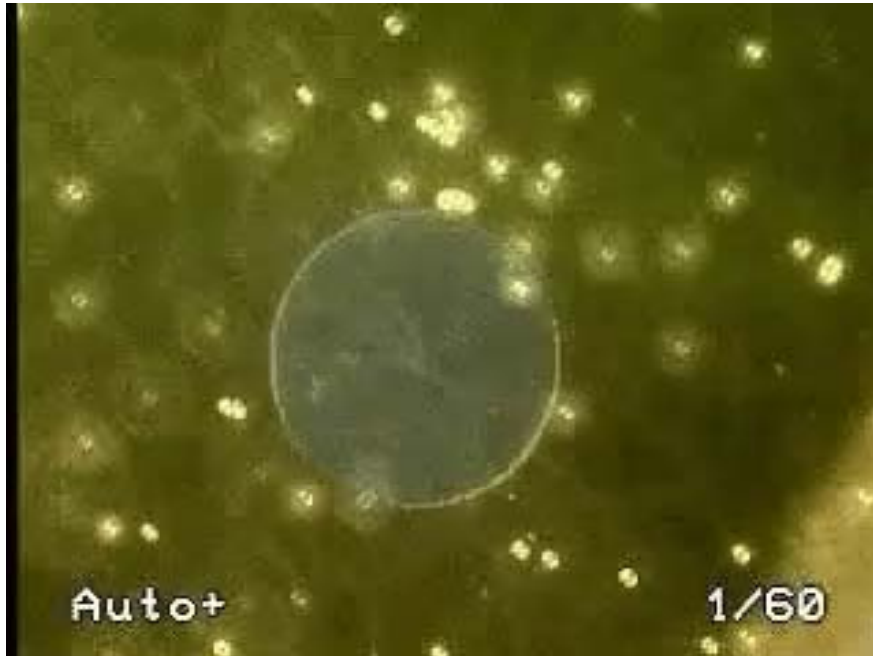
Real-time convective-motion of amidine terminated polystyrene ( 2\ \mu\text{m} ) spheres on Ag patterned gold surface at 500x
