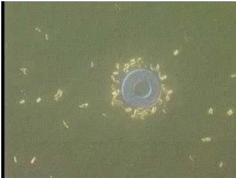
Real-time convective-motion of 2 \mu\text{m} gold rods on Ag patterned gold surface at 500x*
