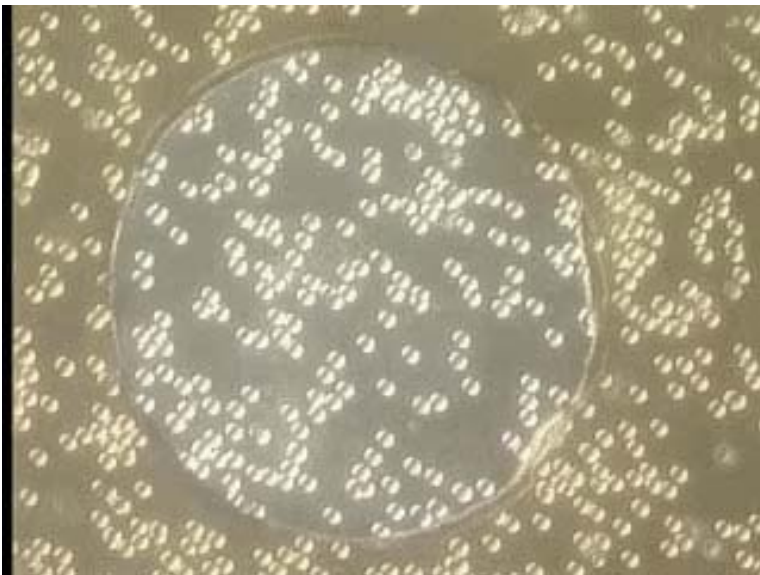
Real-time movie of silica spheres 2.3 \mu\text{m} in diameter pattern formation is now quenched on Ag patterned gold surface at 500x
