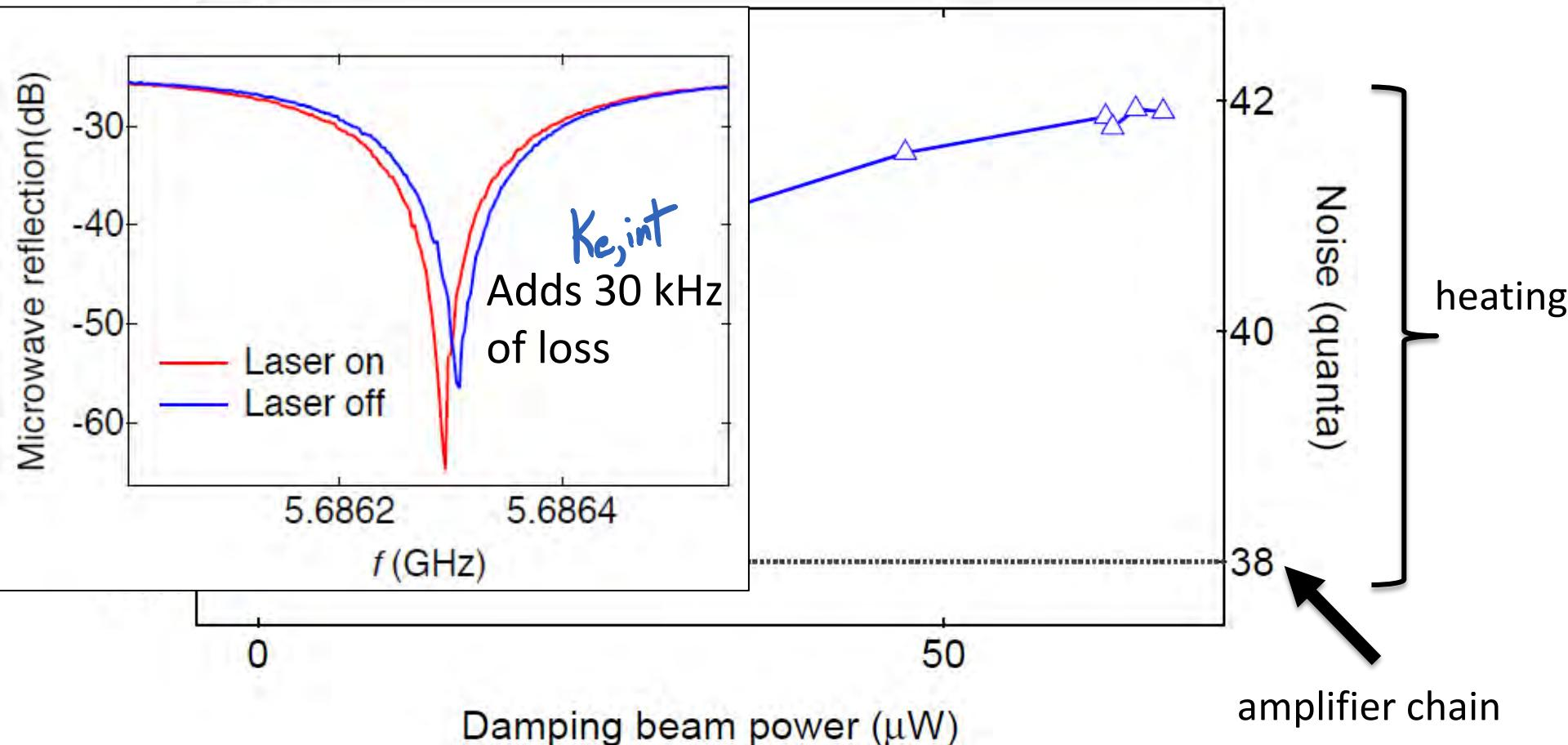
10  $\mu$ W optical power (input) (1 kHz damping) adds 1.5 quanta of noise
