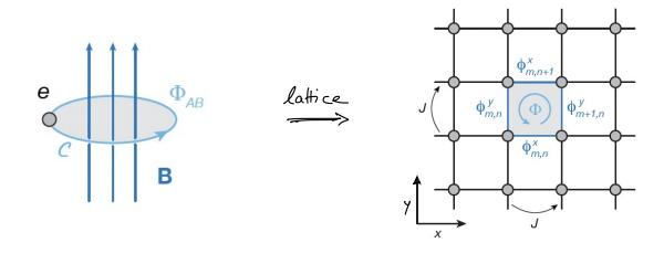
Complex tunneling matrix elements with Peiers phases  $\phi_{m,n}^{i}$ ,  $i = \{x, y\}$ ;  $\phi_{m,n}^{x} = -\frac{e}{t}\int_{m}^{m+1}A_{x}(x, n) dx$
