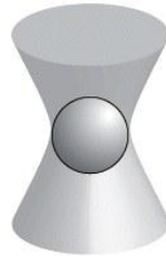
bead pulled to center of an optical trap
