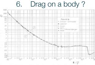
Fig. 1.5. Drag coefficient for spheres as a function of the Reynolds number Curve (1): Stokes' theory, eqs. (6.10); purve (2): Oscen's theory, eqs. (6.13)
