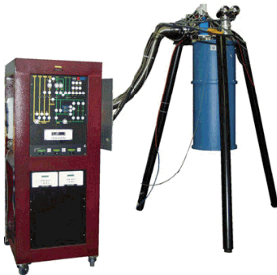
CF refrigerator and gas handling system
