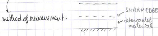
probe after heating and cooling how much the interface blurs ⇔ how much diffusion took place in the sample -
