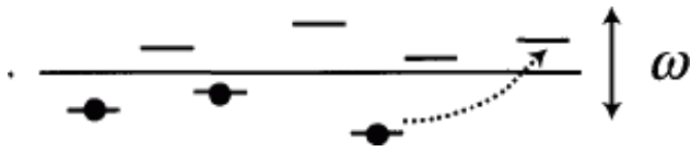
Fig. 9.3. Interpretation of the conductivity in the strongly localized regime. Transitions are absorption of the photons from one occupied localized state to an empty state. This can occur only within a layer \hbar\omega around the Fermi level.
