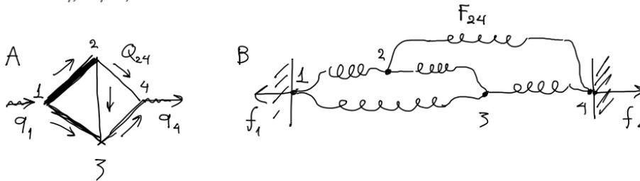
Figure 1: Flow network and its 1D mechanical analogue.
