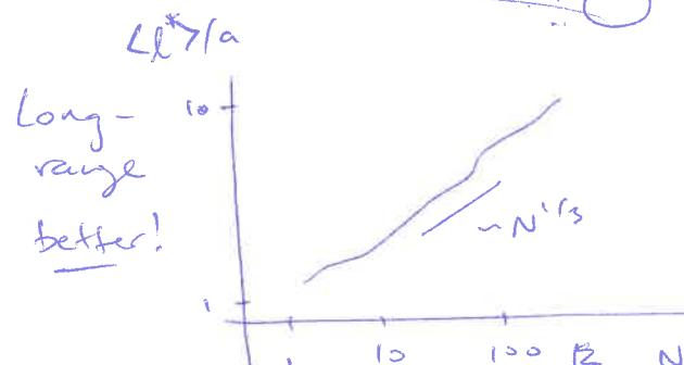
Rationale:  $V \sim N l^{*3} \Rightarrow \epsilon^2 \sim \frac{1}{N^{1/3} l^{*3} c_0 D T} \Rightarrow l^* \sim N^{1/3}$
