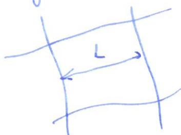
$$\text{Shear modulus } \mu = \frac{k_B T}{L^3} \quad f\left(\frac{\ell_p}{L}\right)$$
